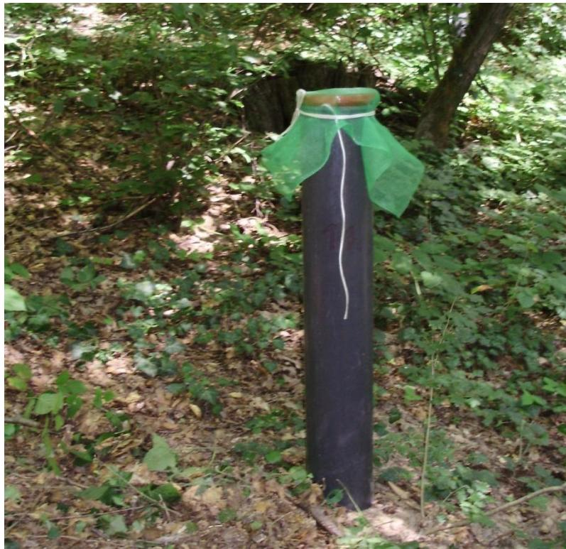
Figure 13. "Throughfall" collector for deposition of perception
